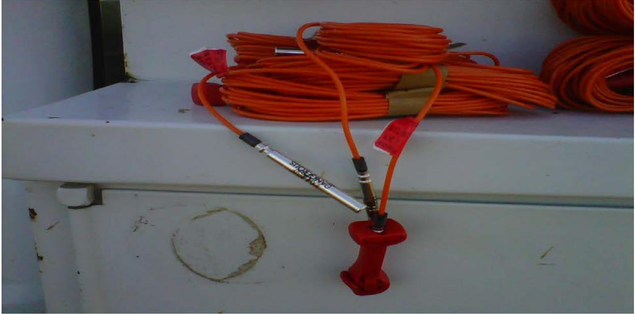
The top picture: Non-Electric Detonators
